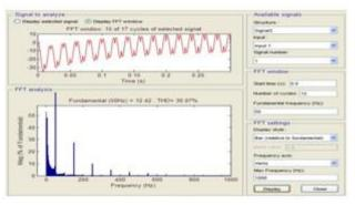
Fig 5 THD for grid connected inverter using Hystresis controller
