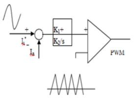
Fig.2. PWM obtained from hysteresis current control
